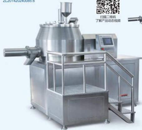
▲ 可换钢型湿法制粒机 Super mixing granulator (Replaceable Pot)
